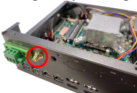
7. And then lock the antenna screw head to the front side of the panel with the hexagonal screw nut ② and tighten it up.
