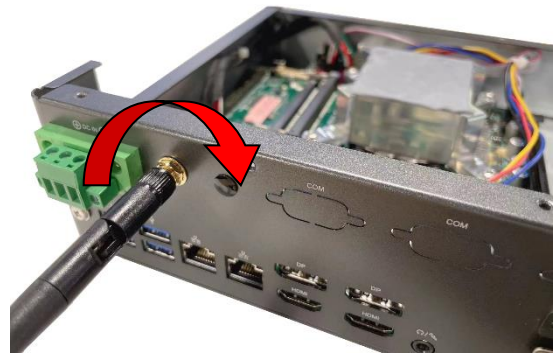
10. Connect the external Wi-Fi receiver antenna to the antenna screw head on the panel.
