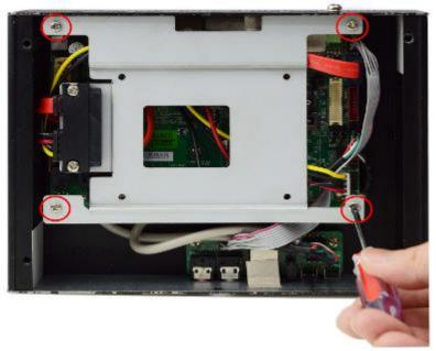
6. Remove the marked screws to dissemble the HDD tray from the system.
