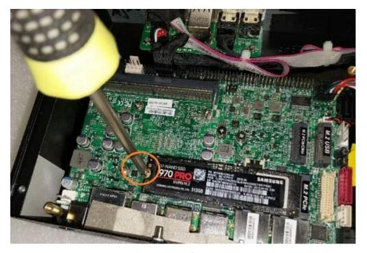
3. Tighten up the screw removed before to the marked spot to secure the card.
