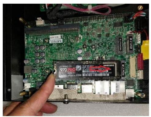
2. Insert compatible M.2 PCle (2280) card into the slot. See to it that the golden-finger side should be fully plugged into the slot.
