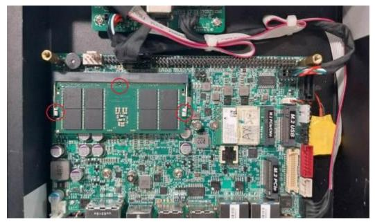
3. Press down to secure the SO-DIMM to the slot. The eject tabs will lock automatically if installing direction is correct.
