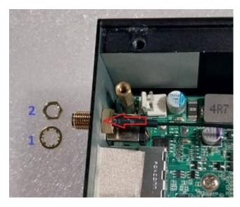
6. Push this antenna screw head into antenna hole of the rear panel from the backside of the panel.
