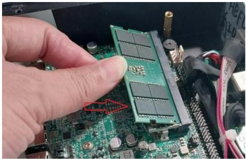
2. Insert the gold-figure side of the compatible SO-DIMM into the slot at a 30 degree angle. See to it that the break of the module fit into the notch of the slot and the golden-finger side should be fully plugged into the slot.
