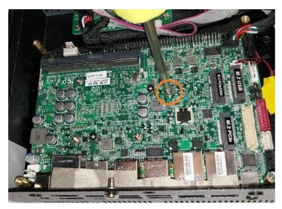
2. Remove the marked screw (MH2) and use it to lock compatible card to the slot in later installation.
