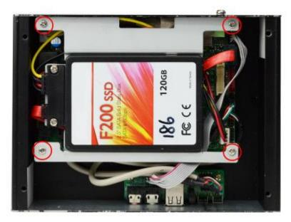
4. Adjust the installed tray as showed above. Fix HDD tray into the system by tightening up 4 screws marked. (refer to I-6)
