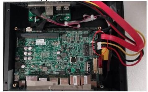
3. Plug SATA power connector and SATA port connector into connectors onboard.
