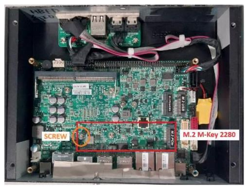
1. Locate the M.2 M-Key PCle (2280) slot on the board. Prepare compatible M.2 M-Key PCle (2280) card. To install compatible card, please remove the screw in the marked spot at first.
