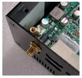
7. And then lock the antenna screw head to the front side of the rear panel with the hexagonal screw nut2 and tighten it up.
