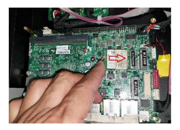
3. Insert the gold-figure side of the compatible card into the slot and press down. See to it that the golden-finger side should be fully plugged into the slot.
