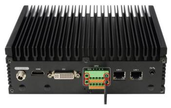
2. Use a screwdriver to remove the screws on the marked spots for further installation. The product showed above comes with two GPIO extension blocks (Plese lock them back to the original positions after wires connection made).
