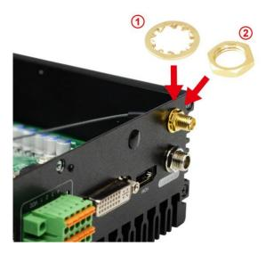
7. And then lock the antenna head to the front side of the rear panel with the hexagonal screwnut 2 and tighten it up.
