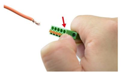
3. Press down the orange key and then insert GPIO wire into the corresponding GPIO socket, as the photo shows.
