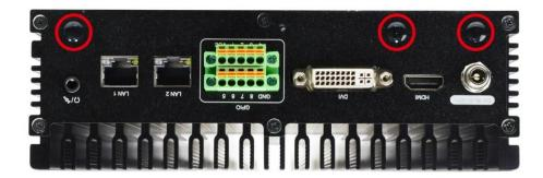
5. Locate the reserved antenna holes on the back panel. Remove the dust-proof plugs on the marked spots from the panel to install the antenna, as the following details show.
