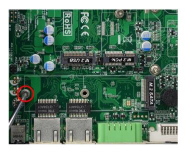
2. The reserved screw is installed in the spot reserved for 2280 card. In the case that you wish to install 2280 card, please remove the screw at first.
