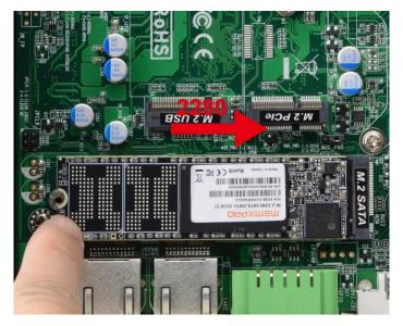
3. Insert compatible 2280 card into the slot.
