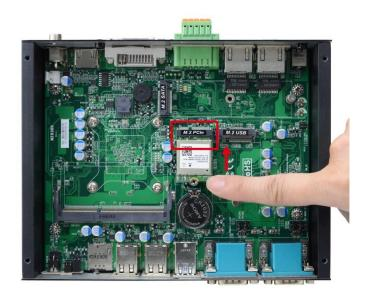
3. Insert the gold-figure side of the compatible card into the slot and press down.
