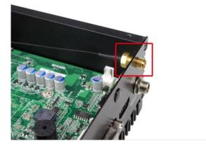
6. Push this antenna head into antenna hole of the rear panel from the backside of the panel.
