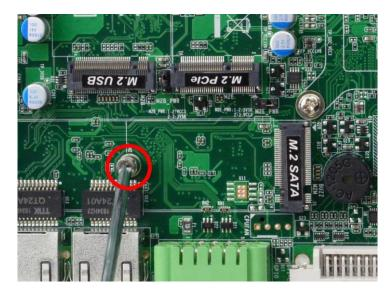
7. Remove the screw at first when you are ready to install 2242 card.
