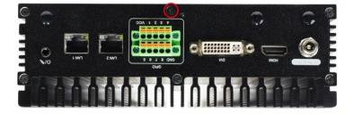
3. Remove the marked screw on the front IO panel.
