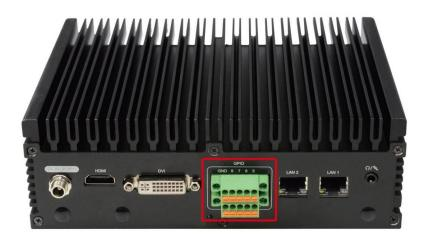
1. Locate the GPIO termial blocks for extension on the front IO panel.
