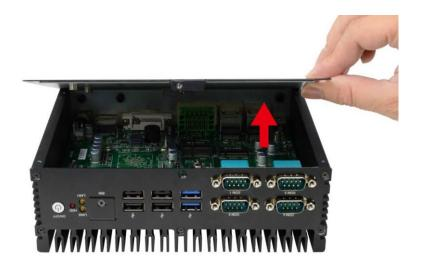
4. Lift the cover up to open the chassis.
