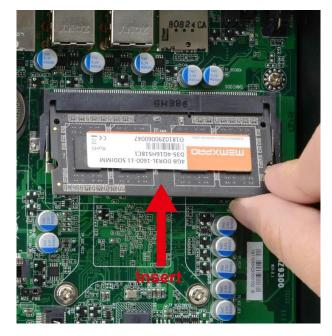
2. Insert the gold-figure side of the compatible SO-DIMM into the slot at a 30 degree.
