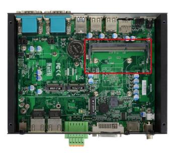
1. Locate the SO-DIMM slot on the board.
