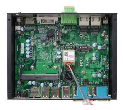
4. Secure the card to the board by tightening up the screw to the marked spot.
