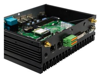
9. The rear panel with antenna heads installed.
