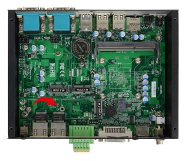
5. For 2242 card installation, please remove the screw and the screw bolt underneath from the default spot MH4 to MH2 at first.
