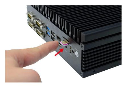
3. Insert the SIM card into the reserved SIM card slot, with the IC side up, as the photo shows.
