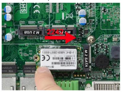
8. Insert compatible 2242 card into the slot.
