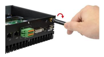
10. Connect the external Wi-Fi receiver antenna to the antenna connector on the rear panel.
