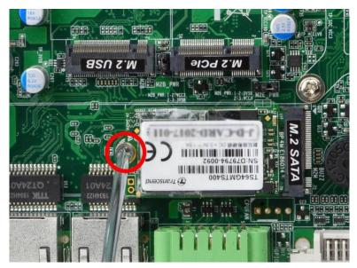
9. Tighten up the screw removed before to the marked spot to secure the card.
