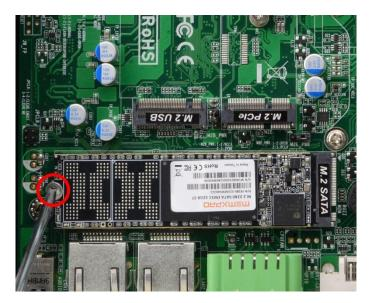
4. Tighten up the screw removed before to the marked spot to secure the card.
