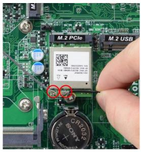
8. Press the metal hat on the end of the antenna string to corresponding antenna slot on the card as shown.
