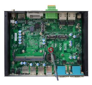
2. Remove the marked screw and use it to lock compatible card to the slot in later installation.
