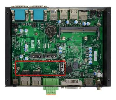
1. Locate the M.2 SATA slot on the board. System supports two types of M.2 card in different lengths (2280/2242). Prepare compatible M.2 SATA card.
