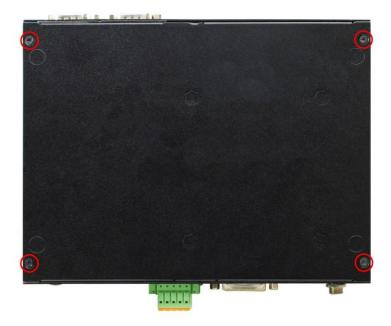
1. Locate the screws at the spots marked on this side of the system and unscrew them one by one.
