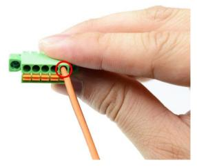
4. Release the orange key to secure the GPIO wire installed, as the photo shows.
