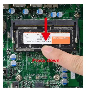
3. Press down to secure the SO-DIMM to the slot. The eject tabs will lock automatically if installing direction is correct.
