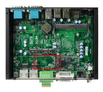
6. Tighten up the screw bolt & attached screw to MH2 spot, as the marked frame shows.
