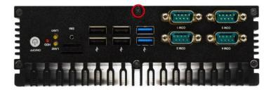
2. Remove the marked screw on the rear IO panel.
