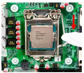
6. Put down the load plate in the direction shown 7. above.
