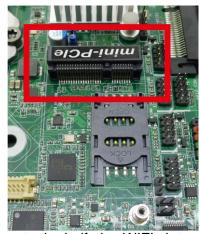
1. Locate the half-size WIFI slot on the board.
