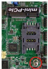
2. Remove the marked screw and use it to lock WIFI card to the slot in later installation.
