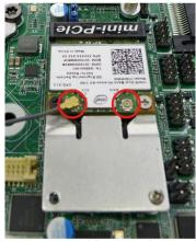
6. Press the metal hat on the end of the antenna string to the antenna slot on the card as shown (If you install two antenna, refer to above steps to finish installation, and press the left metal hat of the left antenna to the left slot, the right metal hat to the right slot).
