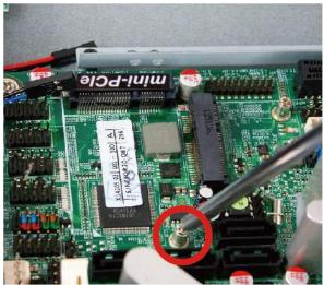
Remove the marked screw and use it to lock Mini PCle card to the slot in later installation.
