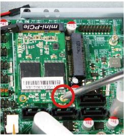
Lock the card to the board by tightening up the screw to the marked spot.
