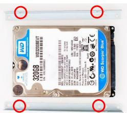
Adjust the HDD and the racks in the directions as the above photo shows.
