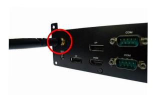
7. Connect the external Wi-Fi receiver antenna to the antenna connector on the rear panel.
