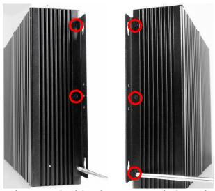
1. Install wall mount rack to the system by tightening two screws in the marked position. Then lock the other three screws on the other side in the same way.
