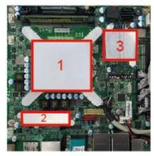
1: CPU Thermal conductive gel (P/N: HCS3XXHS2-F\*1 pcs), 20\*20\*0.5mm
