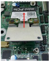
3. Insert the gold-figure side of the compatible WI-FI card into the slot at a 30 degree angle and press down.
