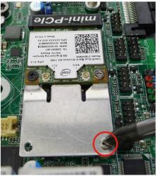
4. Lock the card to the board by tightening up the screw to the marked position.
