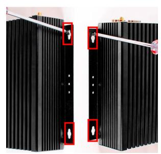
2. Wall mount the system by tightening two screws in the marked positions. Then tighten up the other two screws in the marked positions on the other rack.
