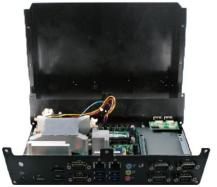
5. Lift the cover up to open the chassis.
