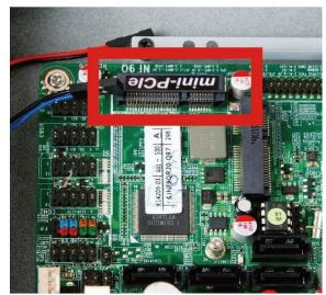
1. Locate the full-size Mini PCIe slot on the 2. board.
