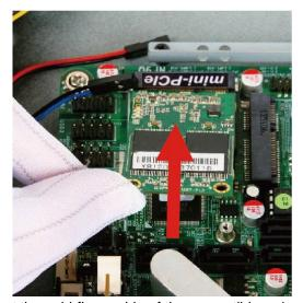
3. Insert the gold-figure side of the compatible Mini PCle card into the slot at a 30 degree.
