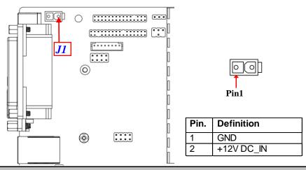
**Warning:** Power connection to Rear **DCIN** and Internal **J1** can not be made simultaneously. Apply compatible power cable to only one of them to power on the system.
