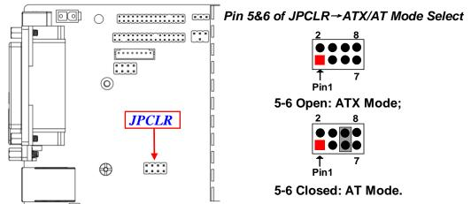
\*ATX Mode Selected: Press power button to power on after power input ready; AT Mode Selected: Directly power on as power input ready.
