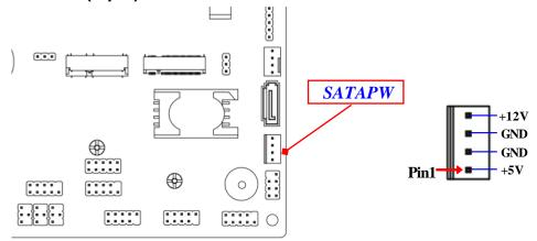
**Warning:** Make sure that Pin-1 of compatible SATA Power out connector is inserted into corresponding Pin-1 of **SATAPW** connector to avoid possible damage to the board and hard disk driver!
