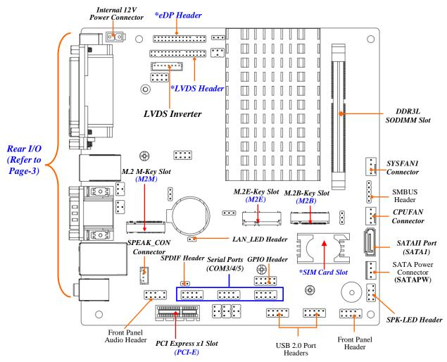
\*Note: 1.The board co-lays LVDS and eDP header; i.e. only one can function at a time. User can go to BIOS settings to select the display output ports. 2. SIM card is supported when M2B (M.2 B-Key 3042) slot is installed with 3G/4G/LTE card.
