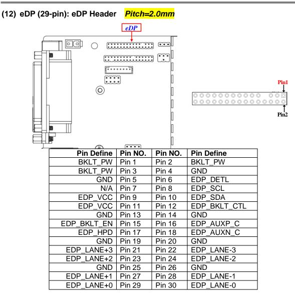
\*Note: The board co-lays LVDS and eDP header; i.e. only one can function at a time. User can go to BIOS settings to select the display output ports.
