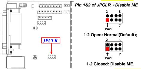
Pin 3&4 of JPCLR (8-pin):Clear CMOS RAM Settings Pitch=2.54mm
