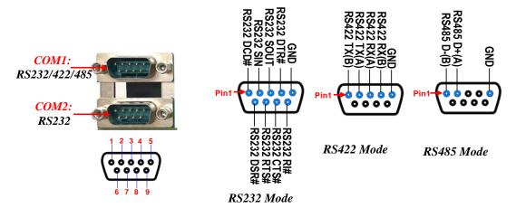
**COM1** port can function as RS232/422/485 port. In normal settings COM1 functions as RS232 port. With compatible COM cable COM1 can function as RS422 or RS 485 port. User also needs to go to BIOS to set **'Transmission Mode Select'** for COM1 at first, before using specialized cable to connect different pins of this port.
