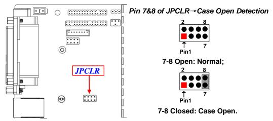
Pin (7&8) short: When Case open function pin short to GND, the Case open function was detected. When used, needs to enter BIOS and enable 'Case Open Detect'
