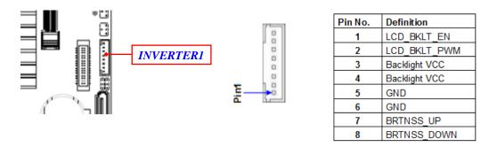
*Warning!* Find *Pin-1* location of the inverter and make sure that the installation direction is correct! Otherwise serious harm will occur to the board/display panel!!
