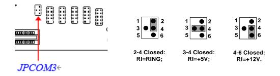
\*Note: Maximum current limit is **500mA** while using 5V or 12V.
