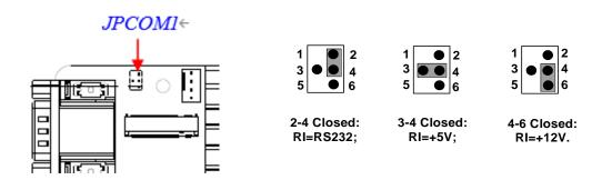
\*Note: Maximum current limit is **500mA** while using 5V or 12V.
