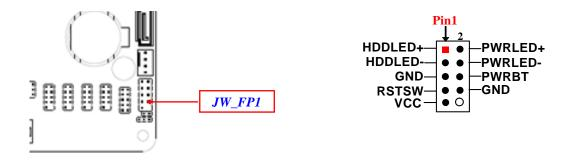
\*Note: Maximum current limit is 1A while using 5V working voltage.
