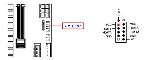
\*Note: Maximum current limit is 500mA x 2 in total while using 5V working voltage.
