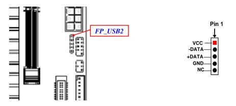
\*Note: Maximum current limit is 500mA x 1 in total while using 5V working voltag
