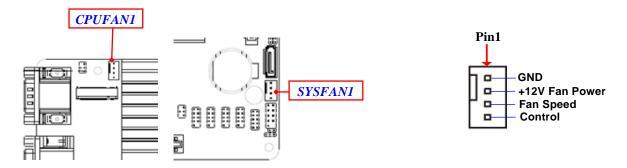
\*Note: Maximum current limit is **1.5A** while using 12V working voltage.
