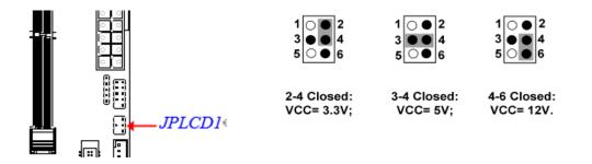
\*Note: Maximum current limit is 2A while using 3.3V, 5V or 12V.
