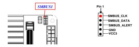
\*Note: Maximum current limit is 500mA while using 3V working voltage.
