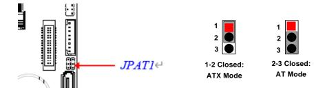
\*ATX Mode Selected: Press power button to power on after power input ready; AT Mode Selected: Directly power on as power input ready. JPM2B1 (3-pin): Power Select (2.0mm pitch)
