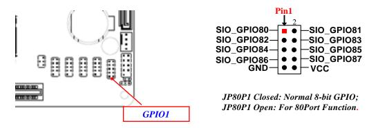
\*Note: 1.Maximum current limit is 1A while using 5V working voltage; 2. Please refer to Page-12 JP80P1 jumper settings for GPIO1 80Port or GPIO Port function select.
